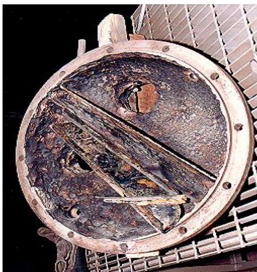
An un coated cast iron end cover after 2 years service
