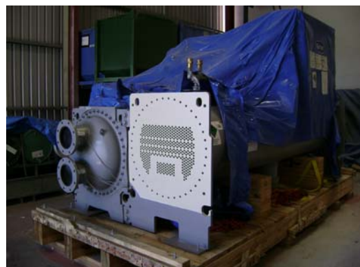
A chiller tube sheet after treatment with Corrocoat VEF
