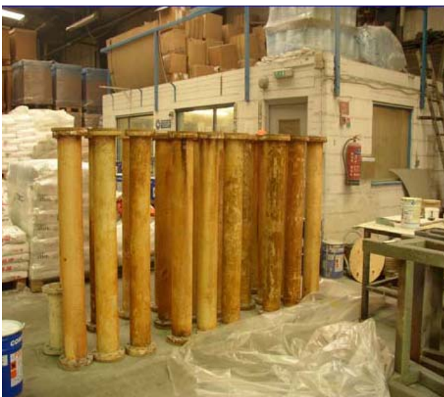
Riser pipes after 21 years in seawater
